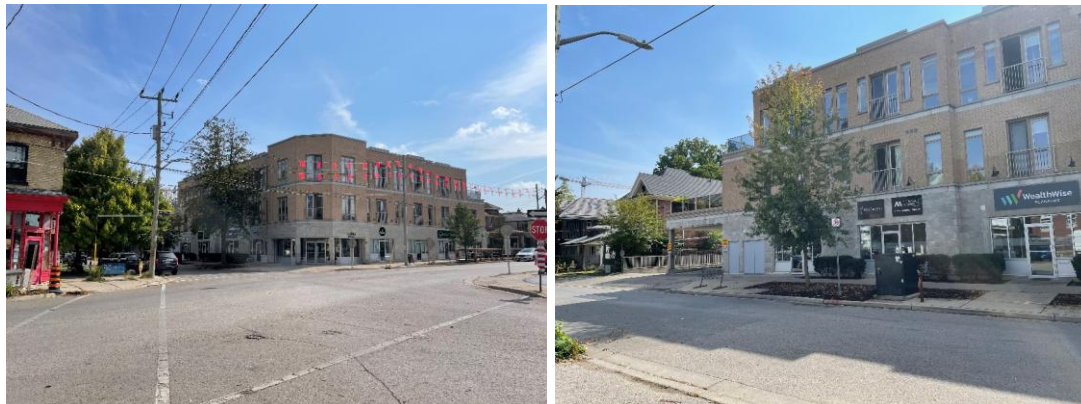
Photo 20 Examples of compatible medium density mixed use development that use brick and stone cladding, have regular fenestration patterns, and provide transitions to adjacent low rise buildings
