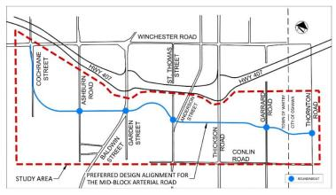
alignment for the Mid-Block Arterial Road has been identified. The preferred design alignment includes a 4-lane cross-section accommodating a multi-use path (MUP) on the north side and a sidewalk on the south side, with 2-lane roundabouts proposed at all intersections except for the intersection at Thickson Road which will be signalized and at Highway 7 which will be signalized when warranted.
