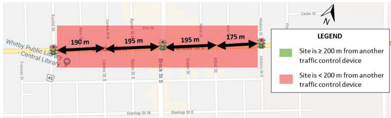
**Figure 13: Traffic Signal Spacing on Dundas Street**
