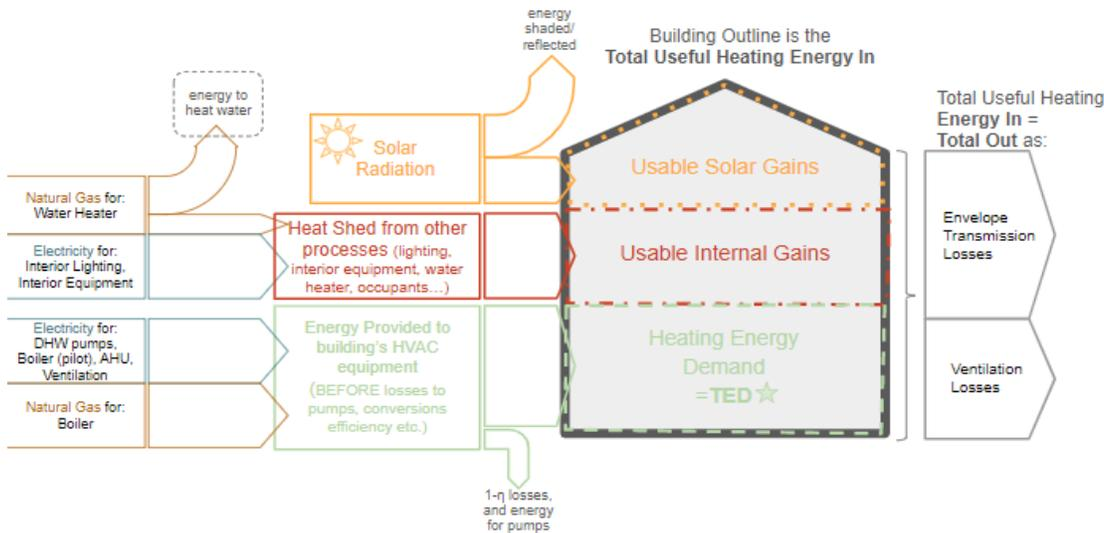
Figure 4. Building energy sub-model schematic.
