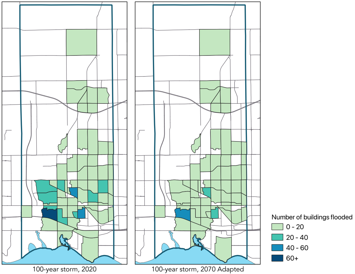
Figure 22. Prevalence of basement flooding by zone in pre-1980s houses for a 100-year flood in 2020 and in the 2070 Adapted Scenario.
